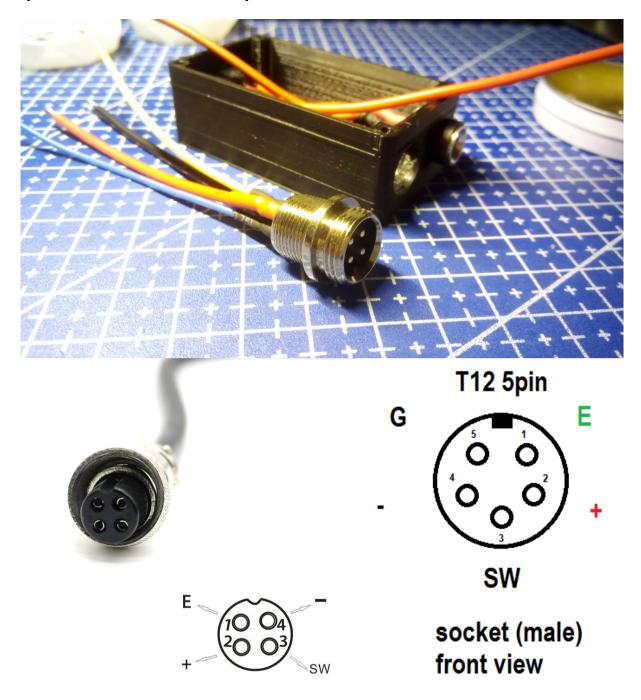
For 5-pin aviator plug connect (G) and (-) together.
